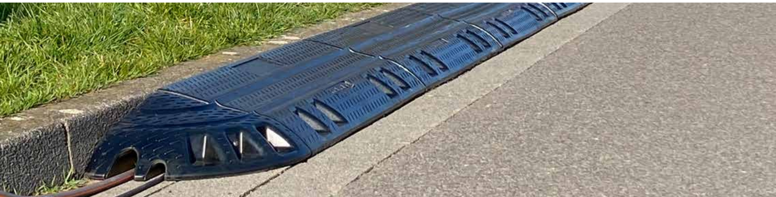
Curb ramp type NOX curb ramp 120 mm high made of recycled material, this ramp can be extended in length as desired and due to the special connection method it is assembled into a solid unit without additional elements – also toolless, the curb ramp has reflective lenses, so that the ramp can not be overlooked even in the dark, the curb ramp can also be provided with a logo sign, so that the ramp is not only functional, but also can be an advertising medium
